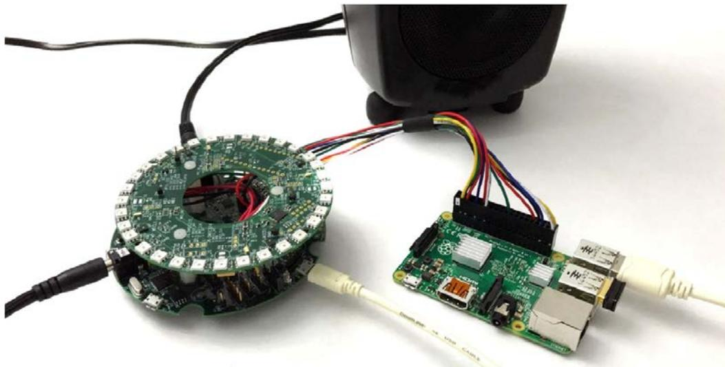
Figure 7. Connecting 5V power supply to J1 connector on the EVK
