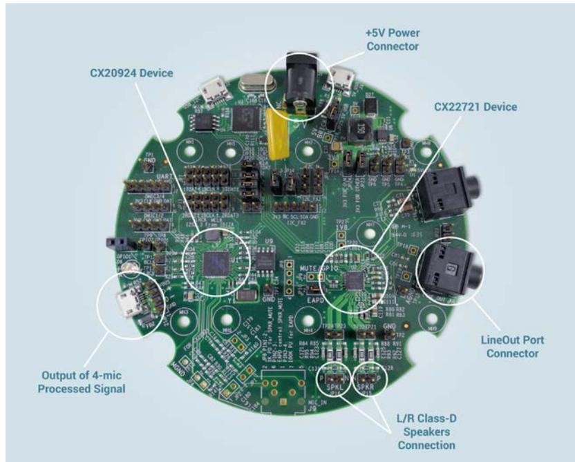
Figure 2. CX20924 EVK: connections, interfaces and devices
