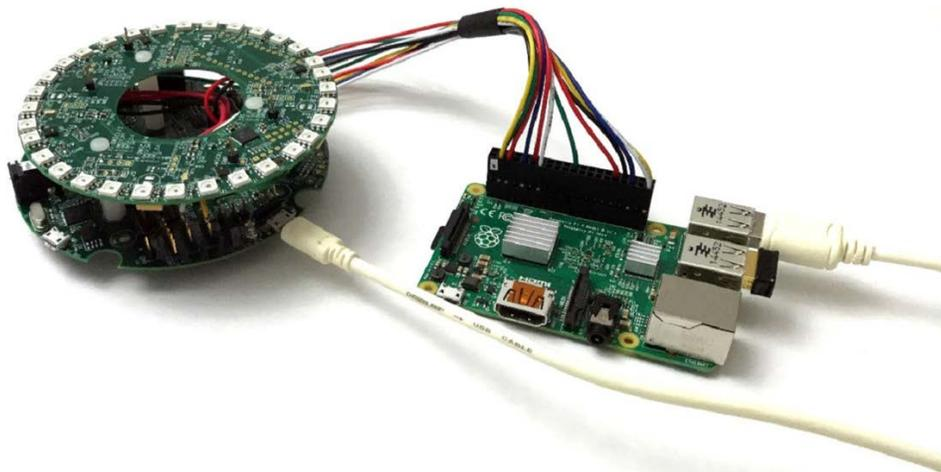
Figure 5. Connecting output of 4-mic processed signal
