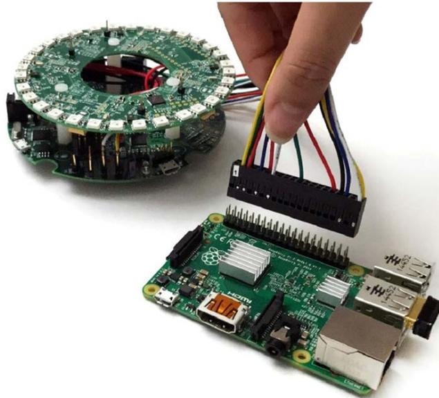
Figure 4. Connecting cable assembly to RPi3 GPIO pins
