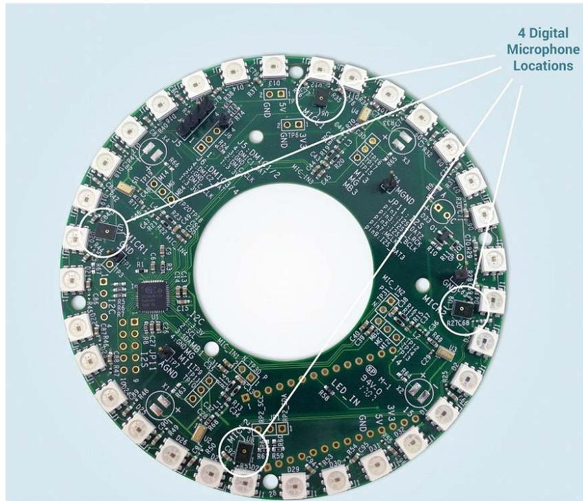
Figure 3. CX20924 Microphone/LED module: four digital microphone locations
