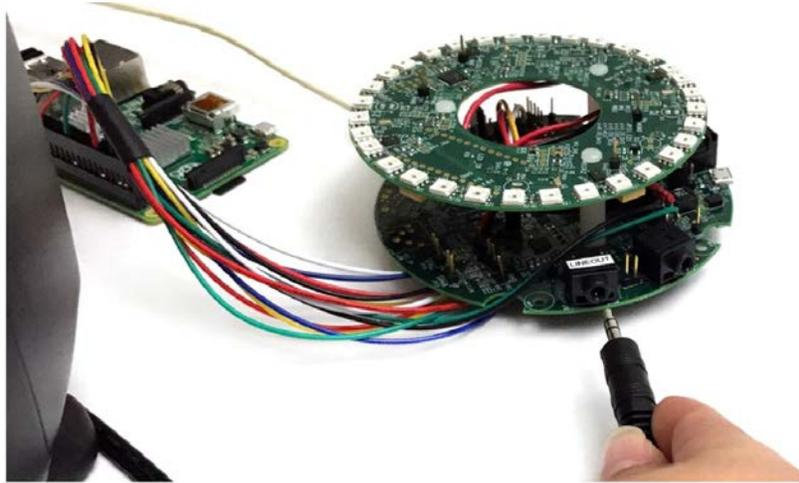
Figure 6. Connecting powered speakers to the LINEOUT port
