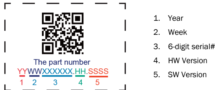
Figure 12. DHAN-S Module Labeling Details
