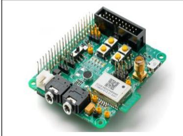
The DHAN-M Expansion Board incorporates a DHAN-M module loaded with either a DECT-ULE Hub (Fixed Part or Base) communication SW stack or a DECT-ULE Device (Portable Part) stack. This platform serves as a development tool for creating application SW running on an external Host MCU.
