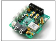
The DHAN-M Expansion Board incorporates a DHAN-M module loaded with either a DECT-ULE Hub (Fixed Part or Base) communication SW stack or a DECT-ULE Device (Portable Part) stack. This platform serves as a development tool for creating application SW running on an external Host MCU. Communication with the Host MCU is either via UART (control. data) and
